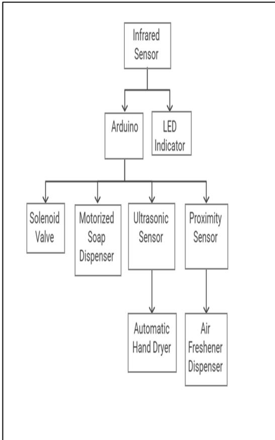
Fig.2: Block Diagram of Touch-Free Restroom
