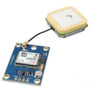
Fig.5 GPS Module NEO6M
