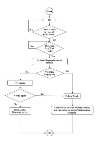
Fig.9 Process Diagram
