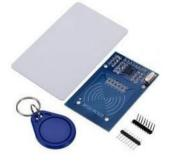
Fig. 4 RFID Reader and Tag
