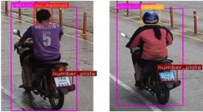
**Fig3.3:** It demonstrates that if a person is not wearing a helmet, the bike's license plate is extracted
