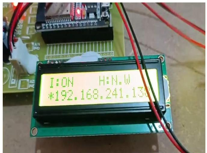
Figure 4.3: Indicating Ignition is ON
