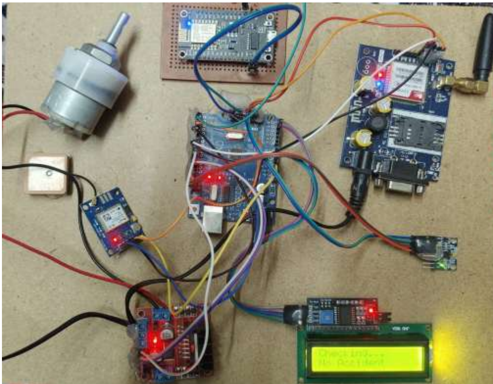
Fig.6. Hardware setup of Smart Automotive Accident Monitoring System
