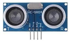
Fig 5. ULTRASONIC SENSOR
