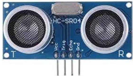
Fig 5. ULTRASONIC SENSOR
