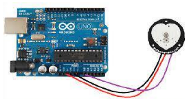
Fig 5 INTERFACING ARDUINO WITH HEART RATE SENSOR
