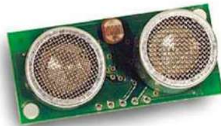
Fig. 3 Ultrasonic sensor SRF08.
