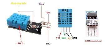
DHT11 is a temperature and humidity device. The sensor comes with an
