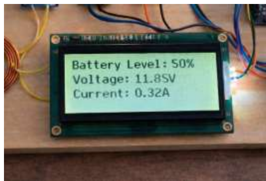
Fig.4 16x2 LCD Display Showing Real- Time Battery Parameters
