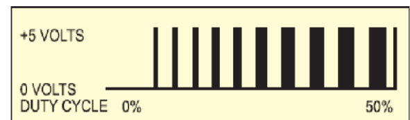
Fig. 2: 5V Pulses With 0% Through 50% Duty Cycle
