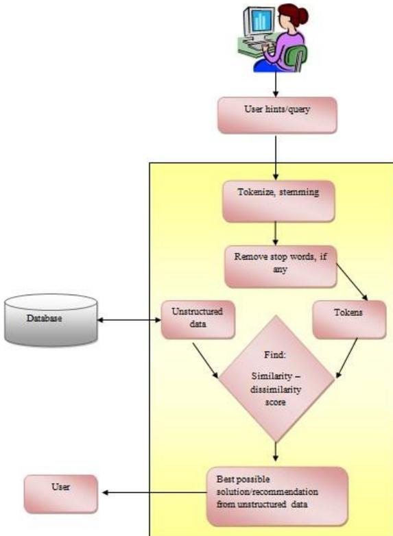
Fig. 2 shows the algorithm-II's flow model for unstructured data.
