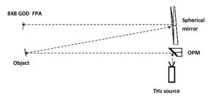
Fig. 2.Experimental setup of the Imaging System.
