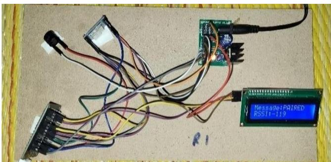
Fig- 14: Receiver 1 (department 1) circuit connection
