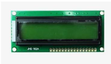
**Fig-7: LCD Display**
