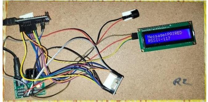
Fig- 15: Receiver 2 (department 2) circuit connection
