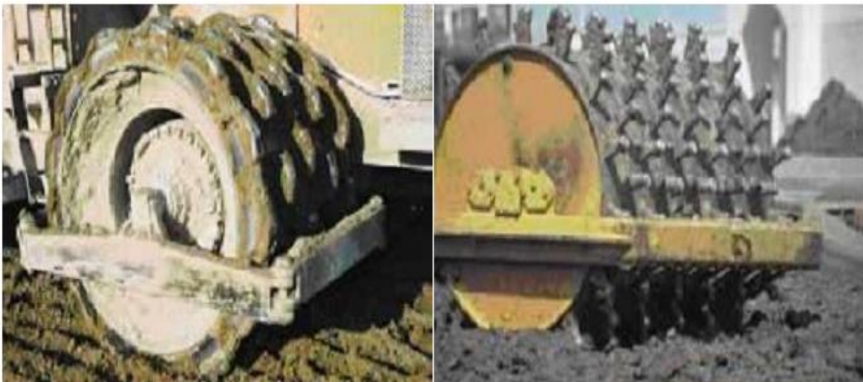
Fig.6 Sheepsfoot (above) & padfoot (below) rollers
