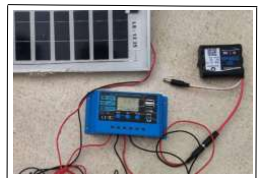
Fig. 6 Solar Panel with Charge Controller & Battery
