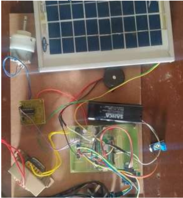
FIG 3 Prototype of Solar Panel and Battery Maintenance Using IOT
