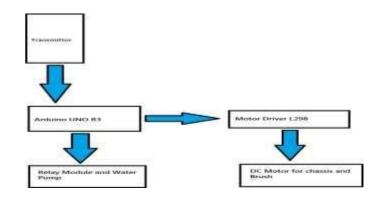
Fig. 1 Solar Panel Cleaner Block Diagram
