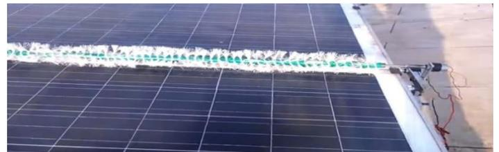
**Fig.3: Roller Mechanism**
