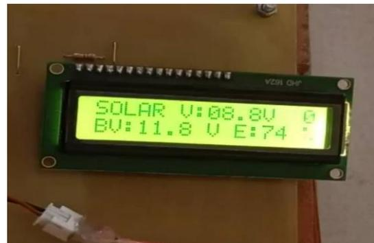
In the beginning we have displayed the message “**WELCOME TO SOLAR PANEL CLEANING ROBOT**” on LCD. After that it displays “Solar Voltage, Battery Voltage and Efficiency of solar panel” before cleaning the solar panels. After cleaning it again displays increased efficiency, battery voltage and solar voltage.
