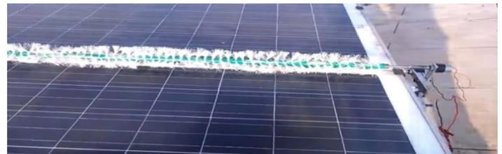
**Fig.3: Roller Mechanism**
