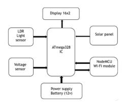
Fig2. Block diagram of solar monitoring system
