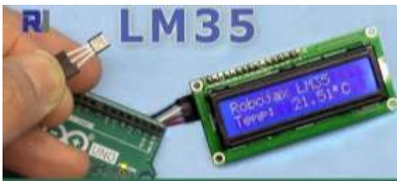
**Fig 7. Temperature Indicator**
