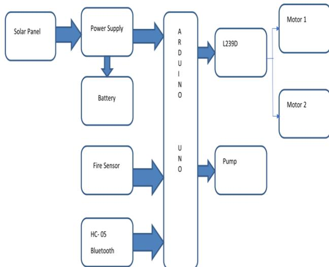
Figure 1: Block diagram of Solar Savior
