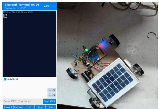
Figure 6: Leftward movement of the prototype
