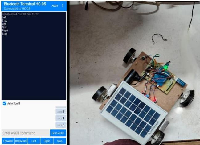
figure 7: Rightward movement of the prototype
