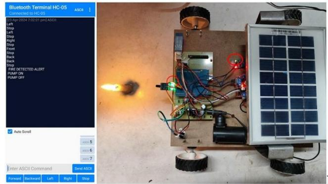
Figure 10: Flame Detection by the prototype
