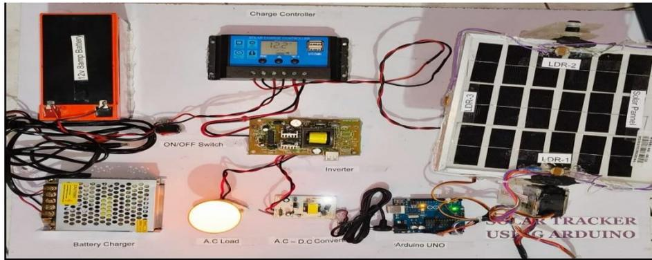
Fig . SOLAR TRACKER USING ARDUINO SOFTWARE
