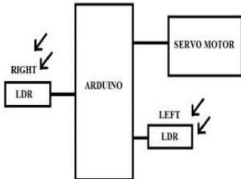
Fig-2: Block diagram
