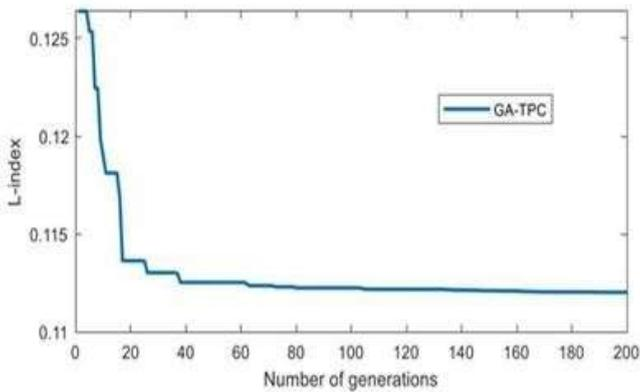
**Fig 2: Convergence Characteristics obtained with 30 Bus System for L-index with TCSC.**
