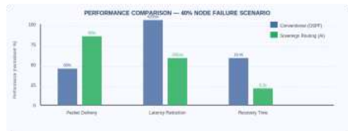
Fig. 6. Performance comparison bar chart: Packet Delivery Ratio, Latency, and Recovery Time for Conventional (OSPF) versus Sovereign Routing (AI) under 40% node failure.
