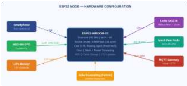
Fig. 4. ESP32 node hardware configuration: smartphone BLE interface, NEO-6M GPS, LiPo power, LoRa SX1276 long-range module, MQTT cloud gateway, mesh peer connectivity, and future solar harvesting.
