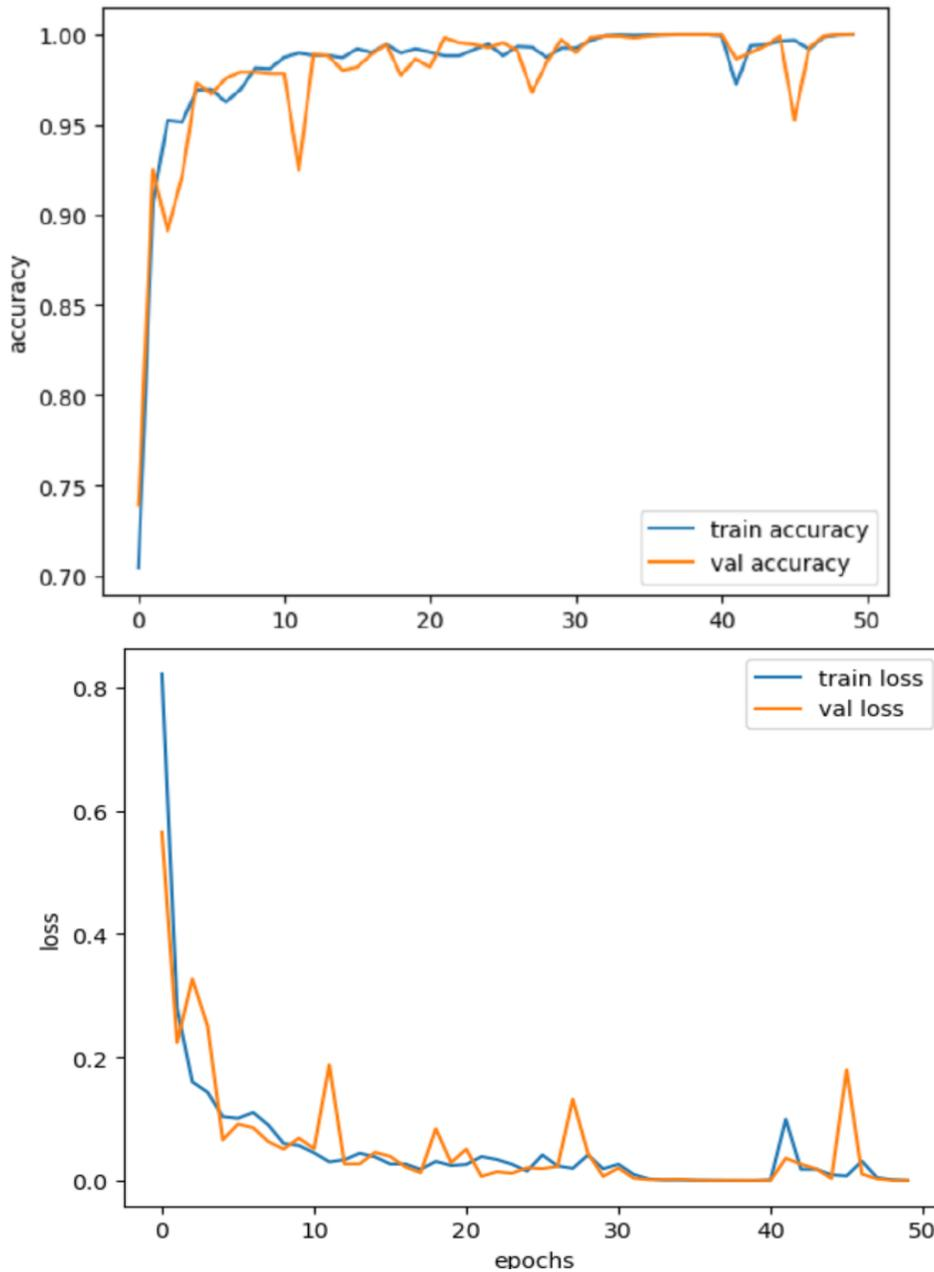
The project followed several steps, including loading the dataset, visualizing the audio signals, extracting MFCC features, splitting the data into training and validation sets and building a deep learning model using LSTM layers. The model was trained for 50 epochs, and the training and validation loss and accuracy were plotted using graphs
