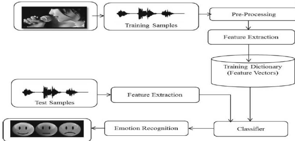
the above figure explains the process of emotion detection using deep learning
