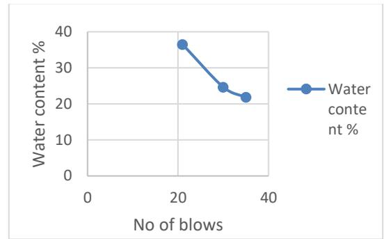
Fig-9: Liquid limit curve for red soil with 1% glass fiber and 40% quarry dust
