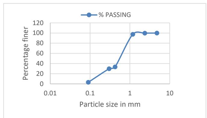
Fig-4: Particle size distribution using sieve analysis for red soil
