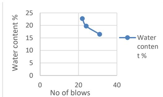
Fig-7: Liquid limit curve for red soil with 0.5% glass fiber and 20% quarry dust
