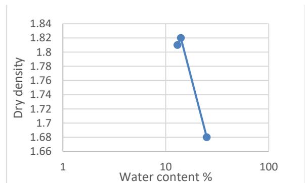
Fig-11: Compaction curve for red soil
