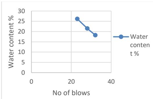
Fig-5: Liquid limit curve for red soil
