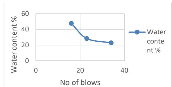
Fig-10: Liquid limit curve for red soil with 1.25% glass fiber and 50% quarry dust
