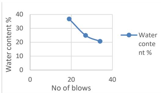
Fig-6: Liquid limit curve for red soil with 0.25% glass fiber and 10% quarry dust
