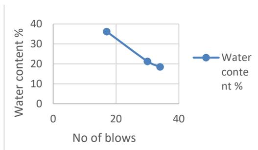
Fig-8: Liquid limit curve for red soil with 0.75% glass fiber and 30% quarry dust
