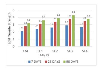
Mix SC3 (84% cement, 10% silica fume, 6% corn ash) achieved the highest split tensile strength at 7, 28, and 90 days. The enhanced performance is due to the combined pozzolanic activity of silica fume and corn ash. Silica fume, rich in reactive
