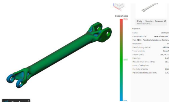
Fig-23: PEKK Drive Shaft stress and displacement
