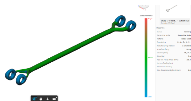
Fig-18: Cobalt Chrome Drive Shaft stress and displacement
