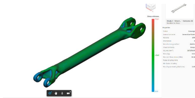
Fig-19: GFRP Drive Shaft stress and displacement
