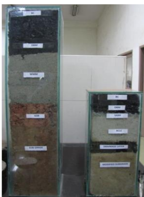
Fig 4 Model of conventional & composite pavement @ LTCRTC
