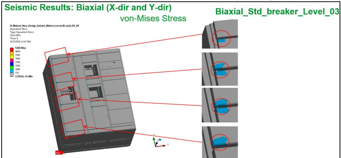
**Peak Stresses are observed on the door hinges of cabinet-1 (encircled in red color). Stresses are more than the Yield limit (235MPa).**
