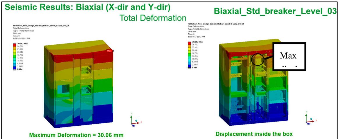
The maximum displacement is observed at the Cabinet-3 outer panel right side location
