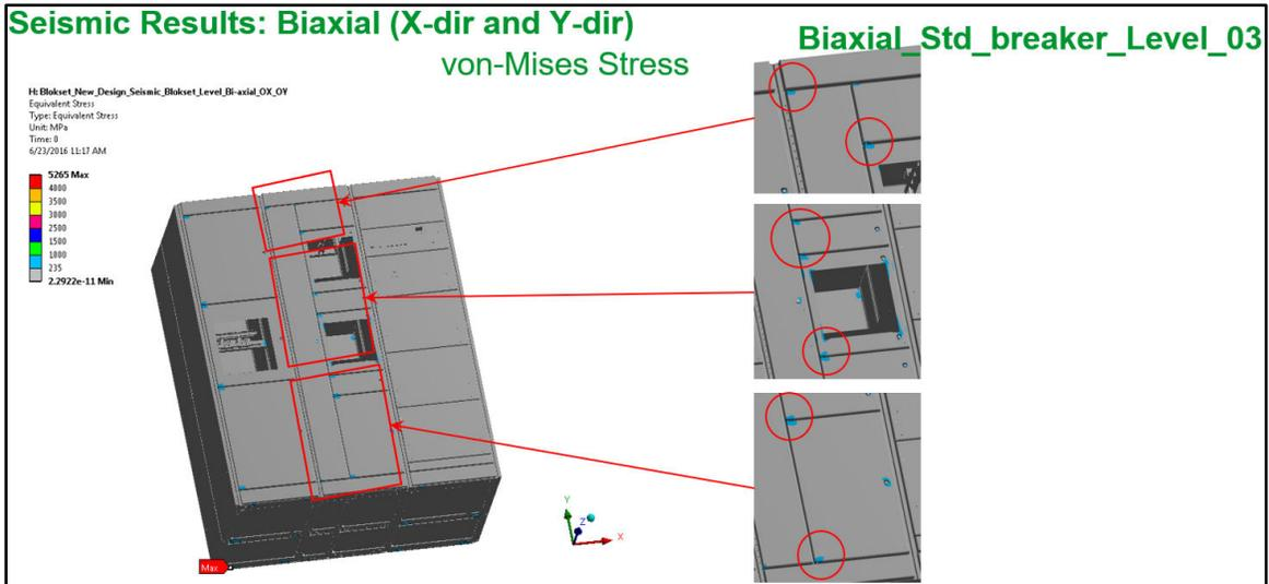
Peak Stresses are observed on the door hinges of cabinet-2 (encircled in red color). Stresses are more than the Yield limit (235MPa)
