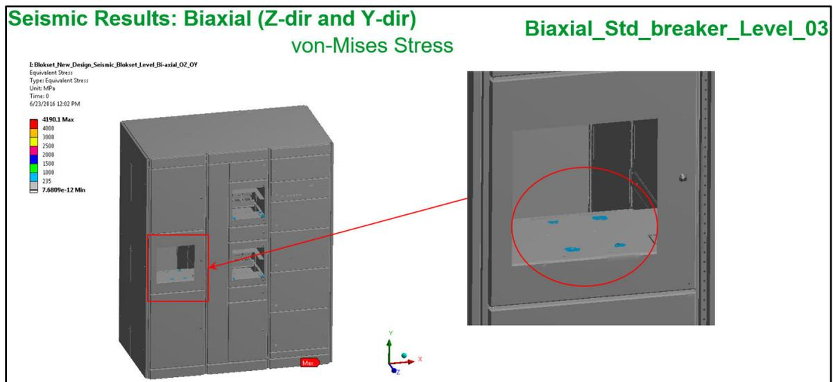
Peak Stress is observed on the fixing of N32 breaker in cabinet-1 (encircled in red color). Stress is more than the Yield limit (235MPa).
