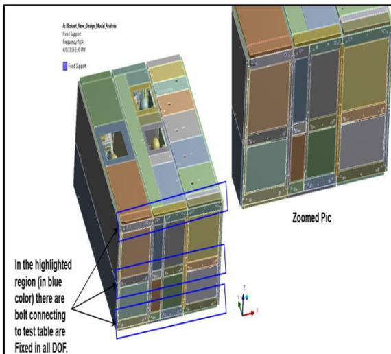
The above figure indicates the location of the masses considered in the simulation. In cabinet-1, we have Device\_N32\_Breaker (location of this mass is shown above) and in cabinet-2, we have Device\_N16\_Breaker (Location of mass is shown above). In Addition to this, we have considered busbar weights as point mass in cabinet-1 = 202.5kg, cabinet-2 = 226kg and cabinet-3 = 60kg respectively. The fixation areas
