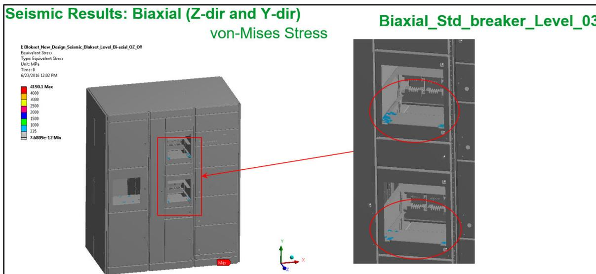
**Peak Stress is observed on the fixing of two N16 breakers in cabinet-2 (encircled in red color). Stress is more than the Yield limit (235MPa).**
