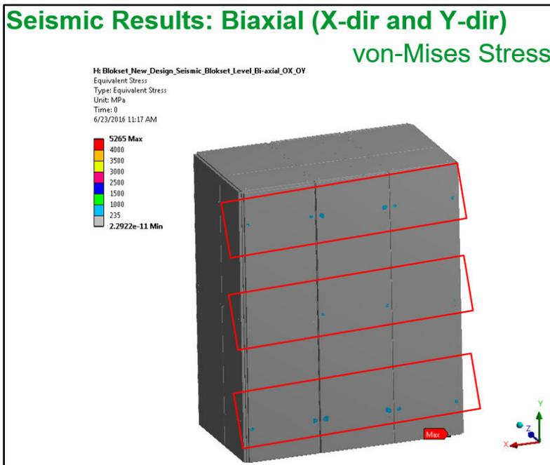
Peak Stresses are observed on the rear panel bolt location in cabinet-1, cabinet-2 and
