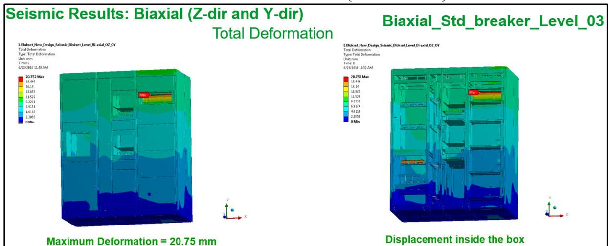
The maximum displacement is observed at the cabinet-3 location (Inside plate)
