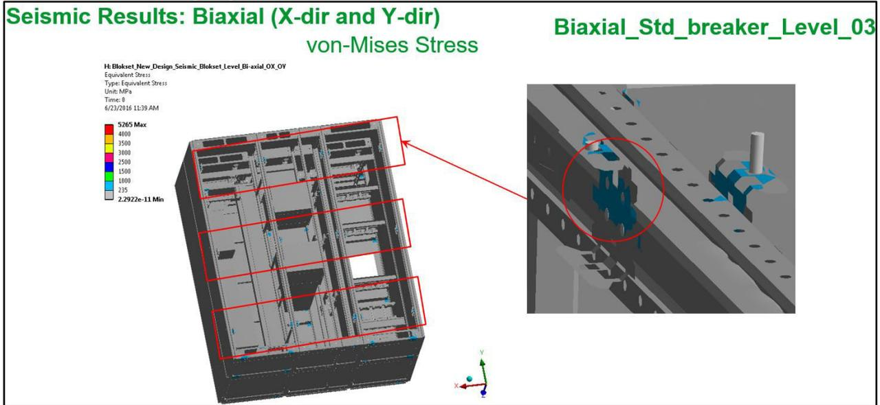
Peak Stresses are observed on the rear panel brackets in cabinet-1, cabinet-2 and cabinet-3 (Highlighted in red color). Stresses are more than the Yield limit (235MPa).
