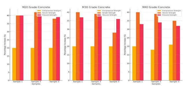
Here the set of bar Diagrams showing the percentage increase in compressive, Tensile and Flexural strength of fiber Reinforced Concrete compared to ordinary Concrete across three samples for each grade (M20, M30, and M40).
