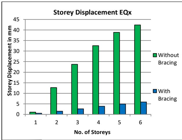
**Fig.1 No. of Storey v/s Storey displacement for Steel Bracing**
