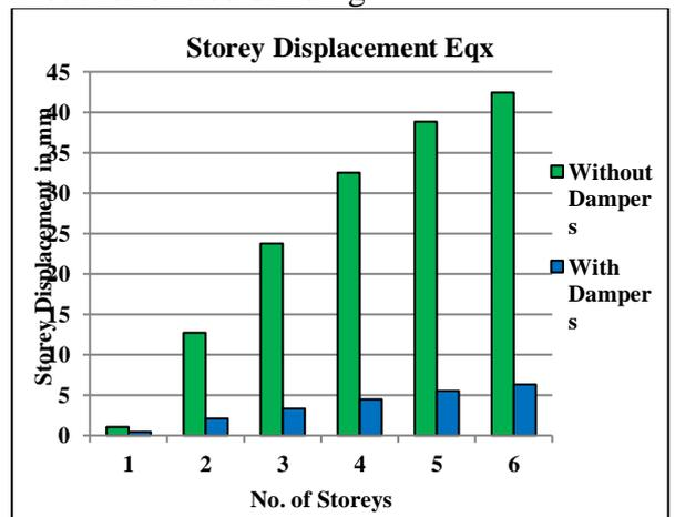
**Fig.4 No. of storey v/s Storey Displacement for Fluid viscous dampers**
