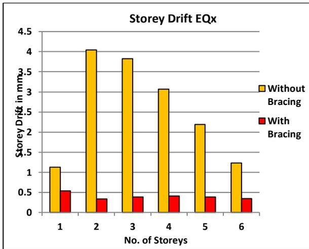
**Fig.5 No. of Storey v/s Storey Drift for Steel Bracing**
