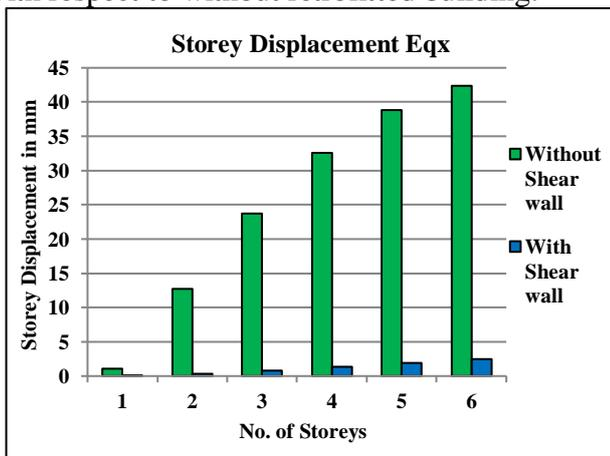
**Fig.2 No. of Storey v/s Storey displacement for Concrete Shear wall**
