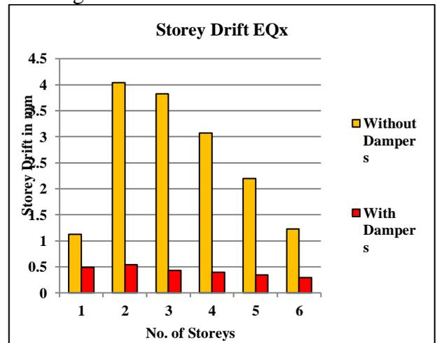
**Fig.8 No. of Storey v/s Storey Drift for Fluid Viscous Damper**
