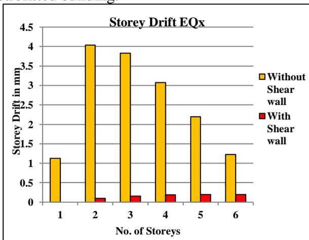
**Fig.6 No. of Storey v/s Storey Drift for Concrete Shear Wall**
