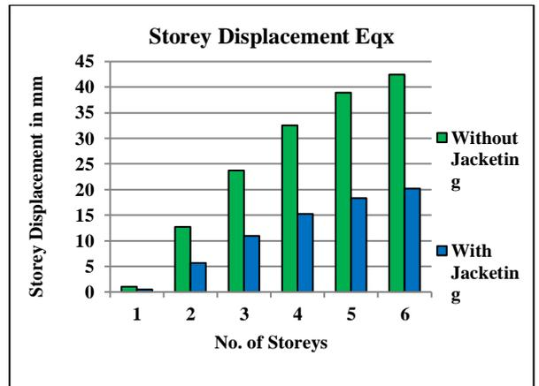
**Fig.4.3 No. of Storey v/s Storey displacement for Concrete Jacketing**
