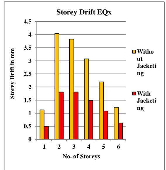
**Fig.7 No. of Storey v/s Storey Drift for Concrete Jacketing**
