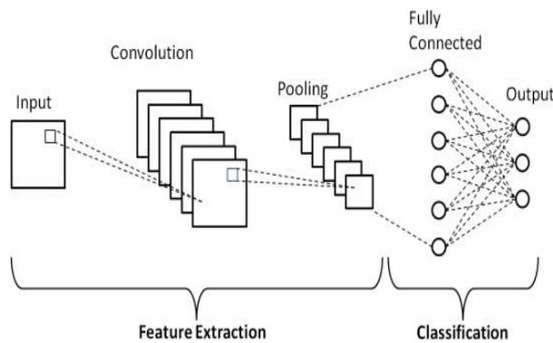
Figure 1. Convolution Neural Network (CNN)
