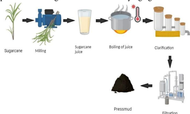
Figure 7 Manufacturing Process of Press Mud
