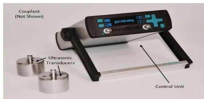
Fig 4.4. Ultrasonic Pulse Velocity
