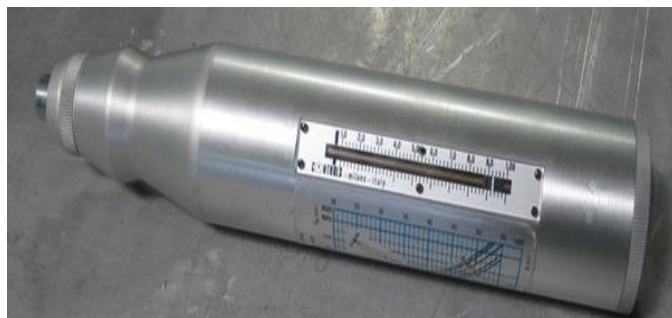
Fig 4.3. Rebound Hammer Test
