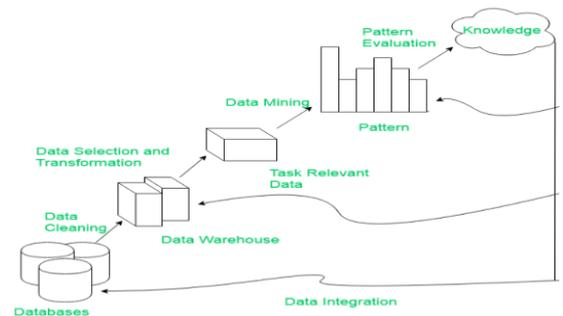
1. Data Cleaning: Data cleansing is described as elimination of noisy and inappropriate information from collection.
