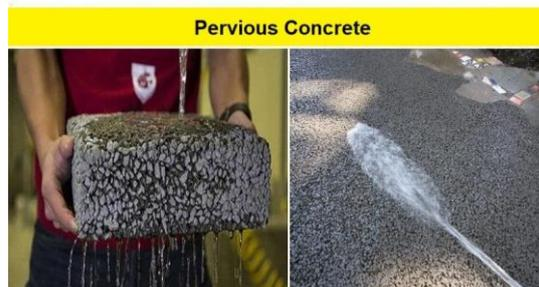
**Fig.2 Pervious concrete vs Conventional concrete**
