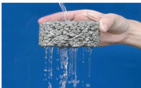
**Fig 1. water percolating through the pervious concrete cube**
