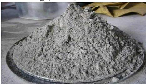
**Fig 4. Ground Granulated Blast Furnace Slag**
