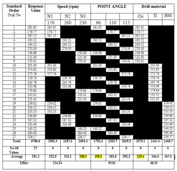
**Cutting forcr Vs Input parameters**
