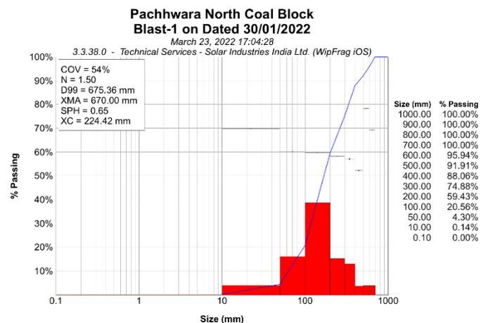
Figure 15: showing the fragmentation analysis of blast-1 (velocity of detonation is 4426 mtr/sec)
