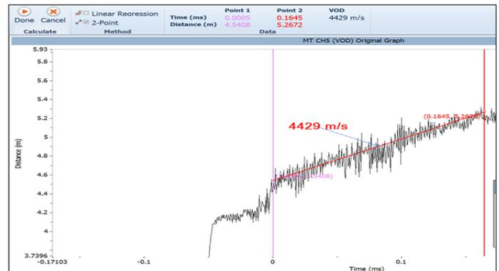
Figure 10: showing the vod analysis of blast- 4.
