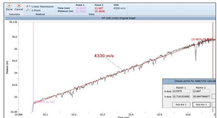
Figure 11: showing the vod analysis of blast- 5
