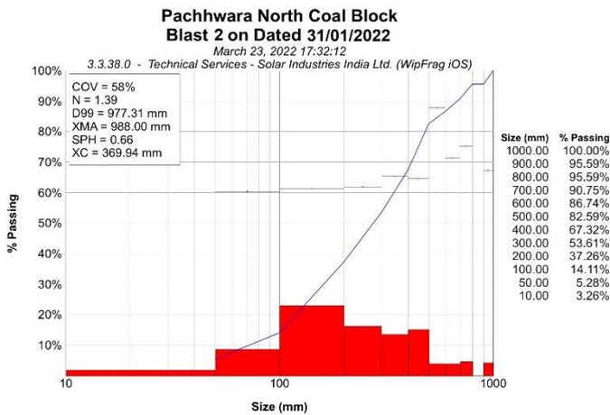
Figure 17: showing the fragmentation analysis of blast-2 (velocity of detonation is 4403 mtr/sec)
