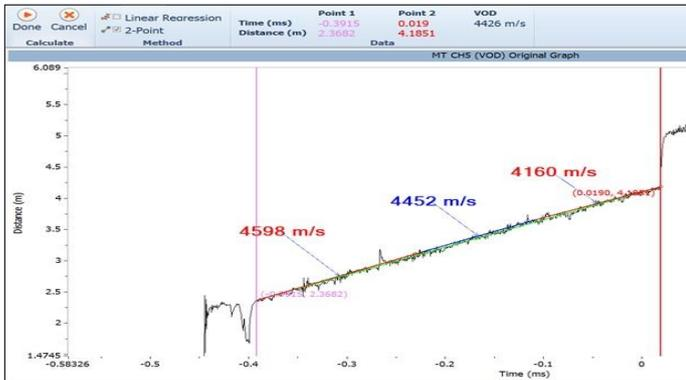
Figure 7: showing the vod analysis of blast- 1
