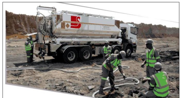
Figure 6: showing the bulk charging at field.
