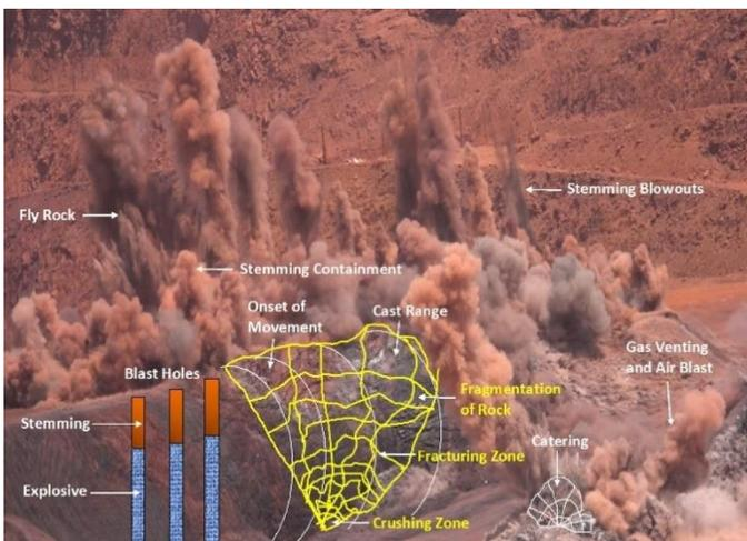
Figure 1: rock- breaking mechanism
