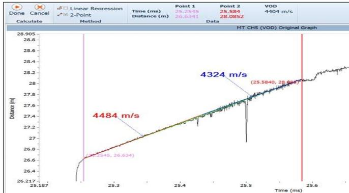
Figure 12: showing the vod analysis of blast- 6
