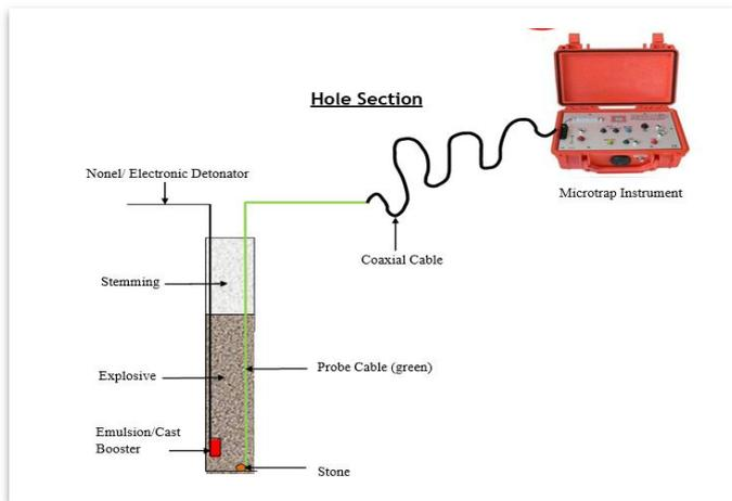
Figure 3: showing the typical model of VOD measurement
