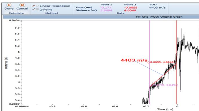
Figure 8: showing the vod analysis of blast- 2
