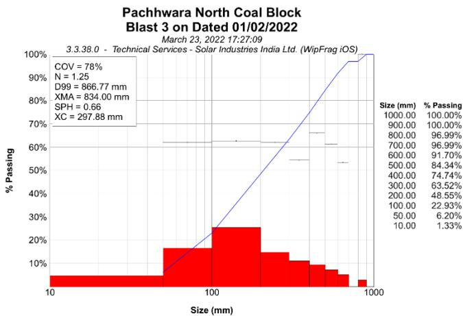
Figure 16: showing the fragmentation analysis of blast-3 (velocity of detonation is 4414 mtr/sec)
