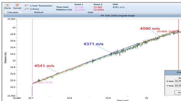
Figure 13: showing the vod analysis of blast- 7
