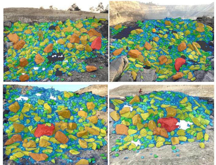
Figure 14: Fragment size analysis at pachwara north coal block with the help of wipfrag software.
