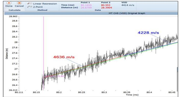
Figure 9: showing the vod analysis of blast- 3
