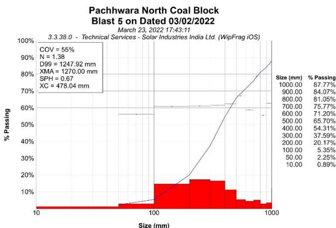
Figure 18: showing the fragmentation analysis of blast-5 (velocity of detonation is 4330 mtr/sec)
