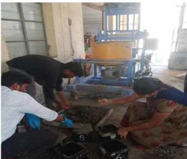
Fig. 6. Casting of concrete specimens
