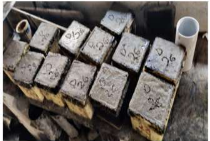
Fig. 7. A view of cast concrete specimens
