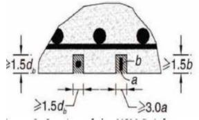
Figure 1.2 Spacing of the NSM Reinforcement (Source: Parth D shahandam (2015))
