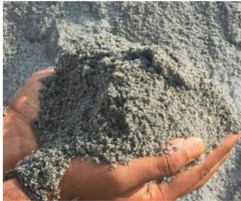
Figure 3.2- Sample of M-sand material
