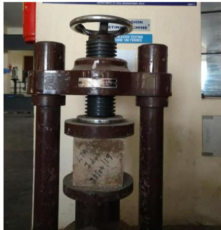
Figure 4.2 – Compressive test of sample cube
