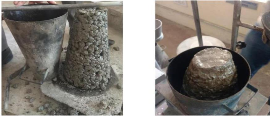
Figure4.1- (a)Slump test (b) Vee Bee test
