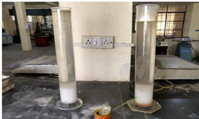
Figure 3.3- Preparation of Alkaline solution
