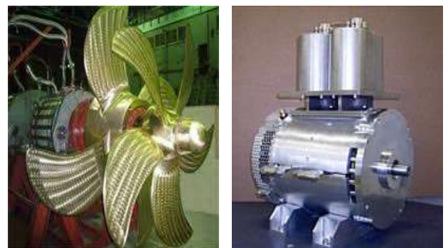
Fig. (f) Superconducting motors Sumitomo: (i) Contra-helical propulsion system (ii) electrical passenger car
