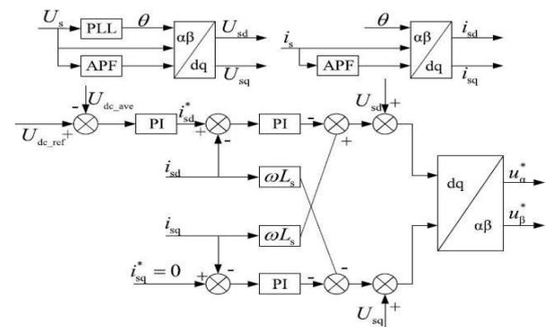
FIGURE 2. Single-phase decoupled current control.
