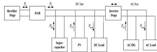
FIGURE 9. Power flows in grid-connected mode.
