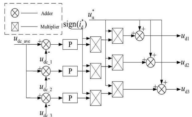
FIGURE 3. Input-stage voltage balancing control.
