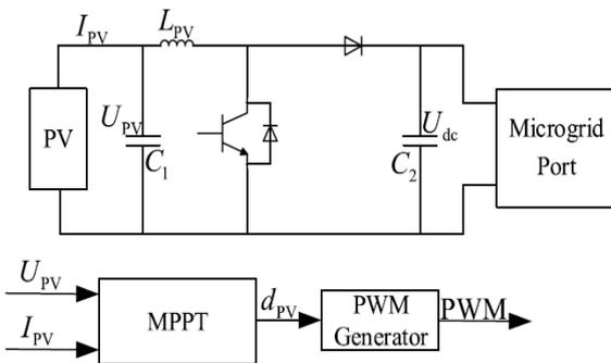
FIGURE 6. Topology and control of the PV DC/DC converter.
