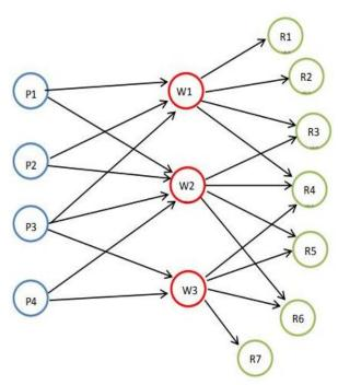
For Example- there are now intermediate transshipment points added between the source and destination. Item being shipped from a plant (P1) must be shipped to a warehouse(W2) before being shipped to the retailer(R2). The graph above shows the transshipment map for a manufacturer of goods. Goods
