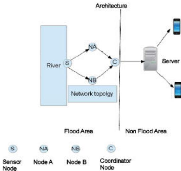
Fig -2: Flood Flood Alert System Model [5]
